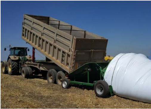
Grain bagger with electric motor is automobile. Thanks to the low receiving hopper, grain can be loaded from dump trailers and rear-loading vehicles.
