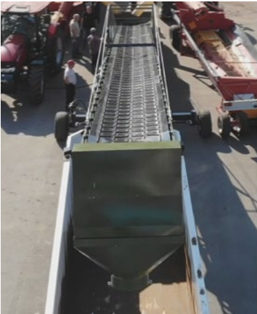
The V-shaped chevron belt 1 250 mm does not damage the seeds
