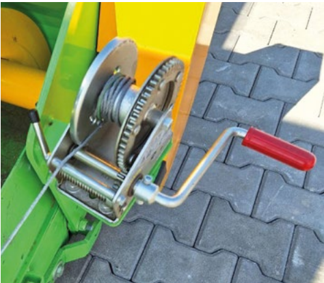
Winch for installing sides
