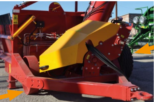
Additional front wheels option for transporting grain in hopper of BNP machine
