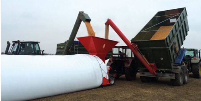
Hydraulically-folding auger GRSH-300/4,5
