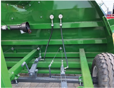
Brake system pressure adjustment for each wheel separately
