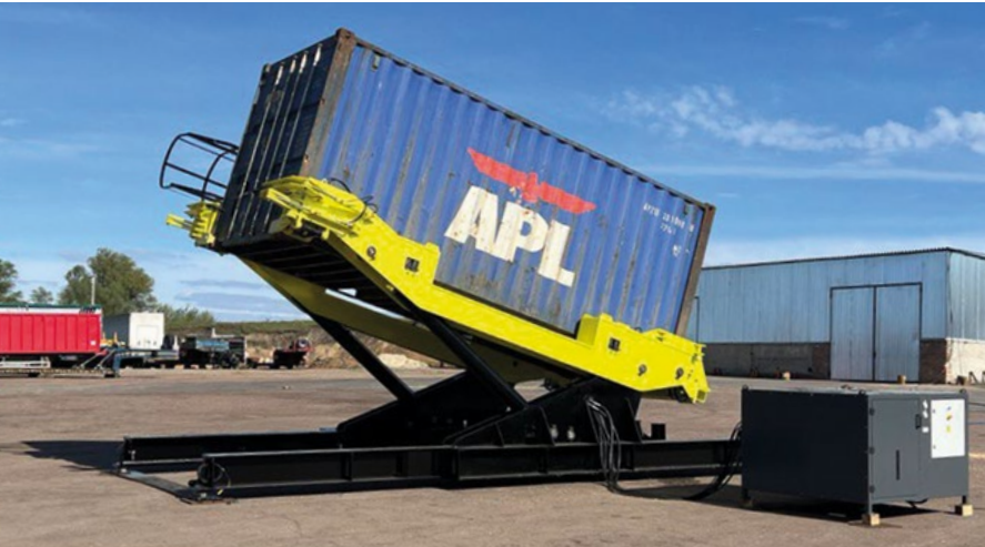
Reinforced hydraulic cylinders for lifting / lowering
