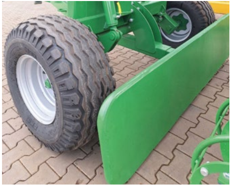
Protective bump what prevent wheels from hitting on bag
