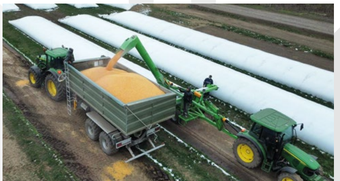
Technology for unloading grain from sleeves into trailers
